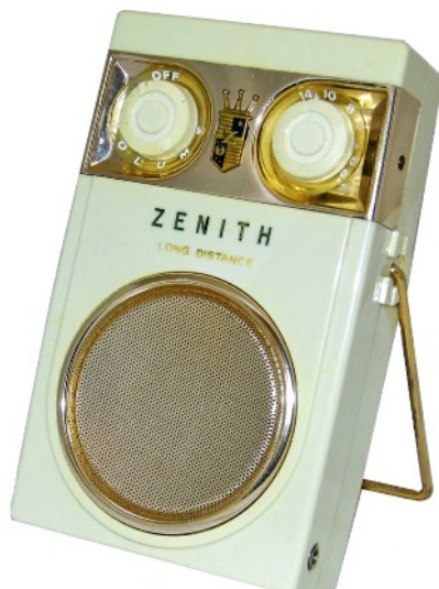
Agents receiver RR-33 was based on Zenith Model Royal 500-D transistor receiver.
